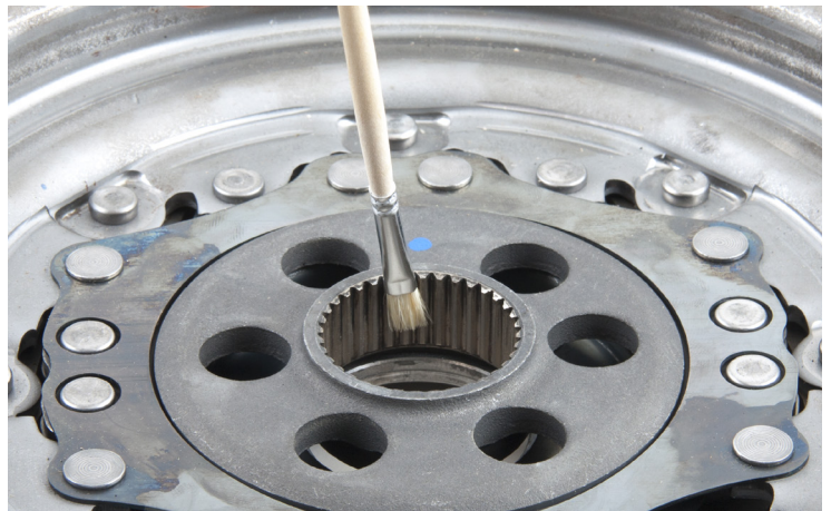
Fig. 1: Some grease should be applied to the inner spline of the DMF every time it is serviced
