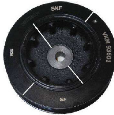
Worn Damper! Needs to be changed!
