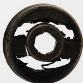
1 Faulty suspension arm bush
