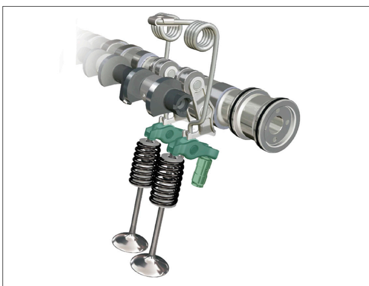
Foto 1: System Valvetronic w BMW
